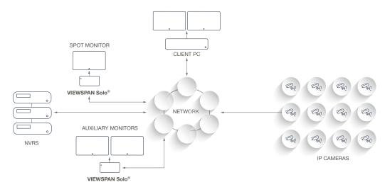
The diagram shows a VIEWSPAN Solo driving an additional spot monitor at an operator workstation and another VIEWSPAN Solo driving a pair of auxiliary monitors elsewhere on the network
