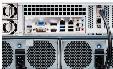
IO PANEL with 4 display port - dual LAN ports - Audio IN/OUT - SAS Expander
