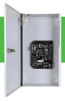
Where a high level of security is required and cabling must be kept to a minimum, the PoE+ DIU 230 offers the ideal solution. Used as part of the AC2000 security management system, the DIU 230 is a complete package that combines Ethernet communication with battery backed lock and door power.
