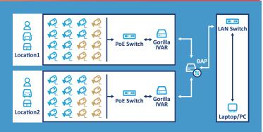
16 channel recording, 6 channel IVA \*5 channel IVA if Face Recognition is used
